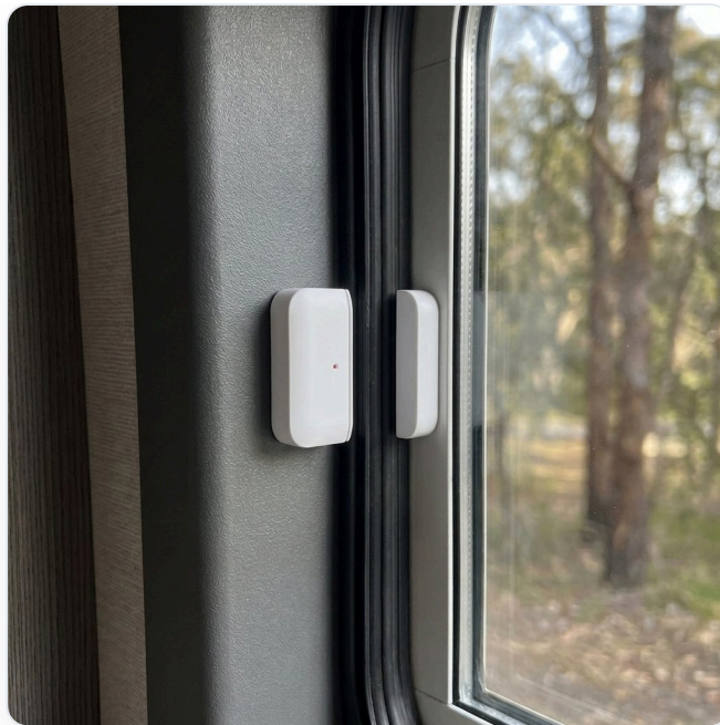
LockSense Pro on a motorhome window: transmitter on the fixed part, magnet on the moving part
